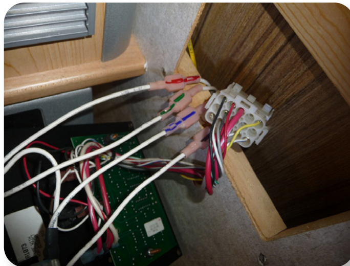
Tracing wires to engineer an added water pump switch
