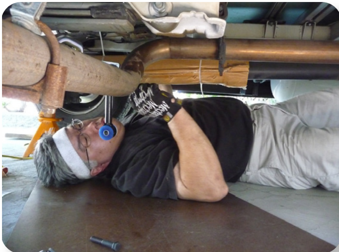
Ellsworth installs an auxiliary sway bar on our Navion
